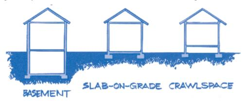
Radon reduction systems can be grouped by home foundation design. Find your type of foundation design above and read about which radon reduction systems may be best for your home.
