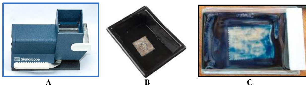
Figure 6: Watermark detections systems: A- is an image of the signoscope used to create the images in Table 1. Image obtained from Worth Point website, B- is a tray containing watermarking fluid. Image obtained from Kenmorestamps.com and C- is the method using blue ink filled plastic pouches. Image obtained from Lynn's Stamp Magazine, Insights "Check watermarks to assure you have the right stamp, April 2021.
