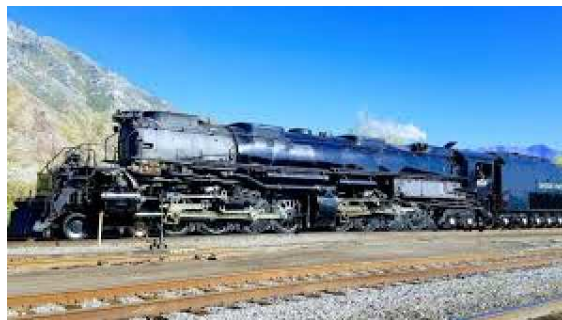
Figure 1: Image of the Union Pacific No. 4014, a 4-8-8-4 "Big Boy" steam locomotive.
