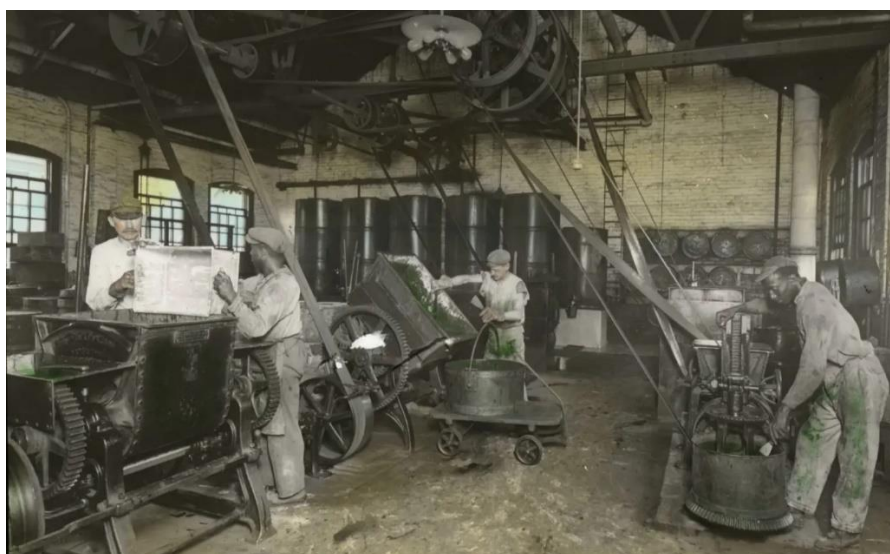
Figure 1: Colorized image of workers mixing ink for the production of stamps at the United States Bureau of Engraving and Printing circa 1914 ( https://unwritten-record.blogs.archives.gov/2016/06/21/engraving-inking-trimming-the-production-of-paper-currency-in-1914/ )
