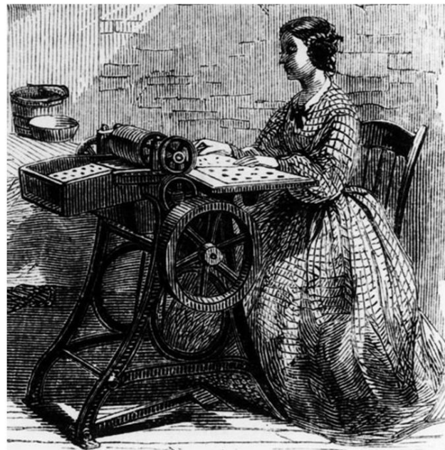
Figure 3: Image taken from https://postalmuseum.si.edu/ showing a rotary perforating machine (circa 1861) with stamp sheets being hand fed into the perforating wheel.
