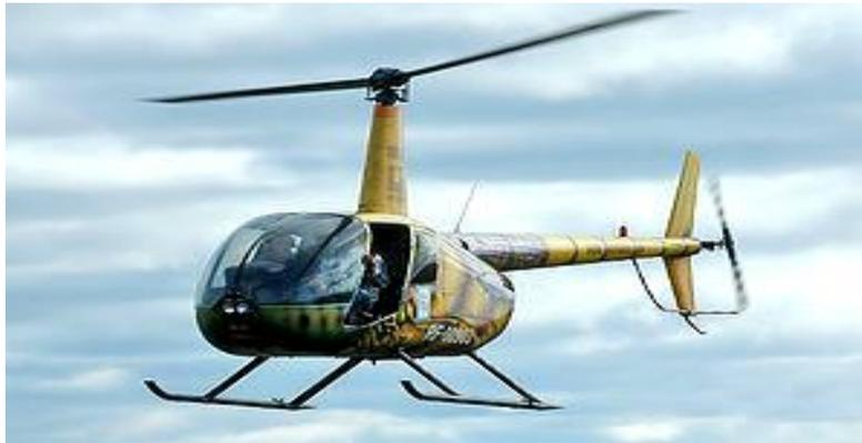
The **Robinson R44** is a four-seat light [helicopter](#) produced by [Robinson Helicopter Company](#) since 1992. Based on the company's two-seat [Robinson R22](#), the R44 features hydraulically assisted flight controls. It was first flown on 31 March 1990 and received [FAA](#) certification in December 1992, with the first delivery in February 1993.
