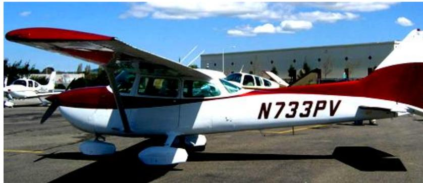
The **Cessna 172 Skyhawk** is a four-seat, single-engine, high wing, [fixed-wing aircraft](#) made by the [Cessna Aircraft Company](#). First flown in 1955, more 172s have been built than [any other aircraft](#).
