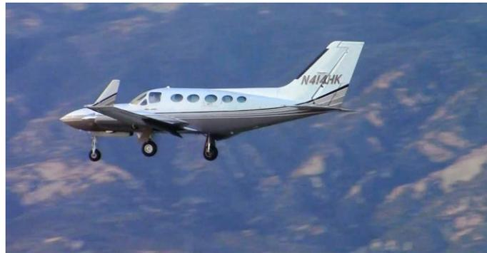
The **Cessna 414** is an [American](#) light, pressurized, twin-engine transport aircraft built by [Cessna](#). It first flew in 1968 and an improved variant was introduced from 1978 as the **414A Chancellor**.
