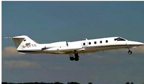
The **Learjet Model 35** and **Model 36** are a series of [American](#) multi-role [business jets](#) manufactured by [Learjet](#). The aircraft are powered by two [Garrett TFE731-2 turbofan](#) engines. Its cabin can be arranged for 6-8 passengers. The longer-range Model 36 has a shortened passenger area to provide more space in the aft fuselage for fuel tanks.
