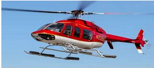
The Bell 407 is a four-blade, single-engine, civil utility helicopter; a derivative of the [Bell 206L-4 LongRanger](#). The 407 uses the four-blade, soft-in-plane design rotor with composite hub; instead of the two-blade, semi-rigid, teetering rotor of the 206L-4. The Bell 407 is frequently used for transport, as an [air ambulance](#), [electronic news gathering](#), and movie making.
