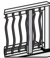
Note: a 2x4 can be used for spacing the Architectural balusters.
