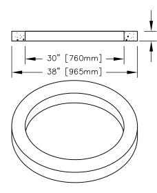
BOTH TYPES OF GRADE RINGS ARE AVAILABLE IN: 2" (50mm) 3" (75mm) 4" (100mm) THICKNESSES
