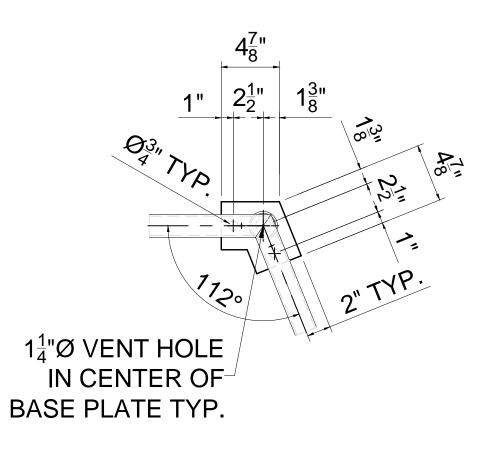
$\frac{\text{DETAIL C}}{\text{SHAPED BASE PLATE ASSEMBLY}} \\ \frac{\text{P5 - PLATE } \frac{1}{2}" \text{ X 4" X 4 } \frac{7}{8}"}{\text{TYP. @ L/H & R/H POSTS}}$
