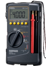
CD800a Digital Multimeter (600 V)
