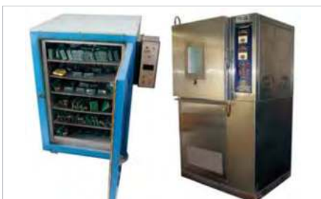
Environmental Chamber To Simulate -20°C to 100°C (Rh upto 100%)
