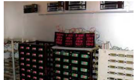
Burn-In at 55°C to Ensure Stability
