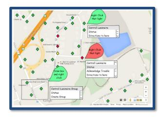
current, condition, etc. Each luminaire can be administered individually, or as one of many configurable groups. Dimming cycles can be programmed and downloaded, or immediate control of any luminaire can be exercised. Future Special Event control programs can be constructed and propagated to a selected group of luminaires
