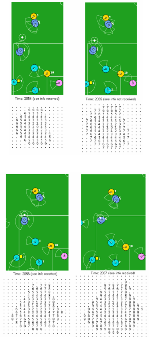
Fig. 2. Our teammate with number 7, adjusts map’s positions of opponent with number 7, using “see” information received.
