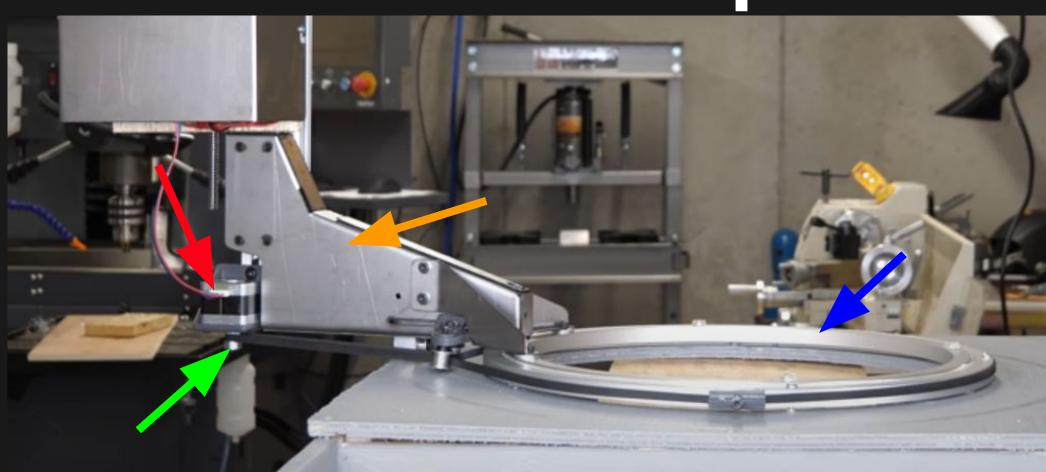
The motion in the main mechanism was heavily inspired by this one that is much more complicated and precise. This design came courtesy of the youtube channel "Stuff Made Here". This design uses a stepper motor on a massive carriage to drive a belt which moves his part around the users head. Mine includes the same concept of using a belt that wraps around a large ring. However, mine is made out of PLA plastic, and uses a DC motor rather than a stepper motor.
