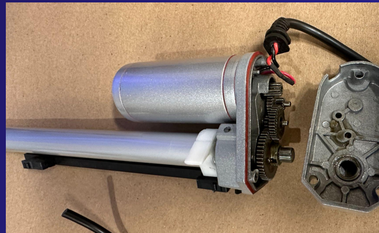
Disassembled actual linear actuator to see inner workings. Reverse engineering.
