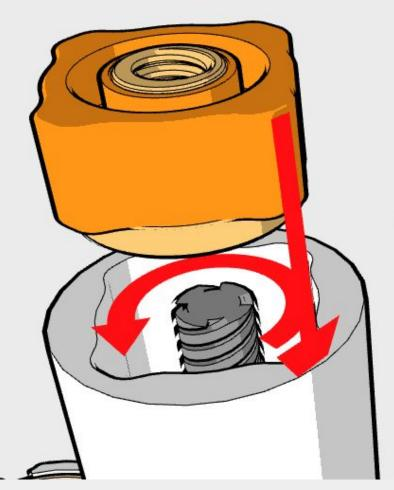
Step 7: Turn on motor, and align/press the lead screw coupler onto the lead screw.
