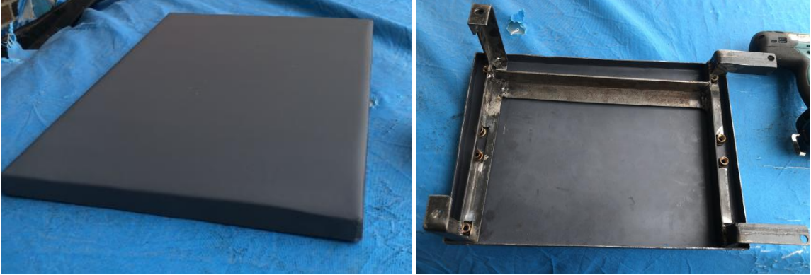
Figure [7]: Battery Tray (Top View) and (Bottom View)
