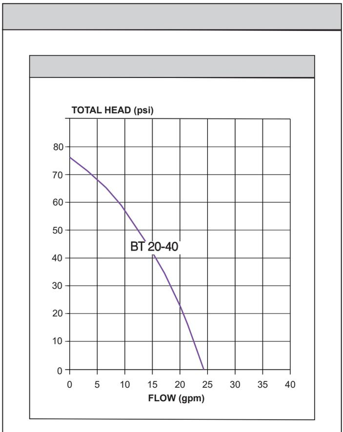
Add incoming pressure to maximum pump boost for shut off pressure.
