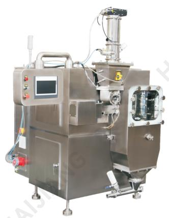
This equipment has a strong adaptability for all kinds of material, can be used to produce the desired mesh granules according to the different needs without any additive during the granulating. With easy process, high batch capacity and easy cleaning etc, it is widely used in pharmaceutical, food and chemical industry.
