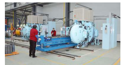
氢碎炉 Hydrogen decapitation furnace
