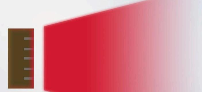
Without optical shaping, the beam diverges rapidly
