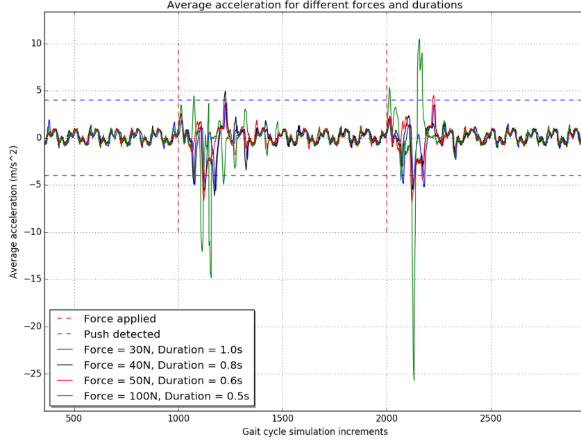
Figure 3.13: Force detector tested with combinations of different forces and durations
