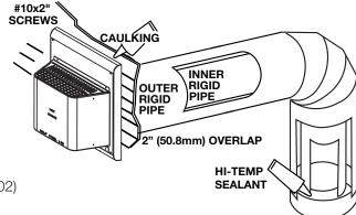
C. Insert the vent pipes through the firestop maintaining the required clearance to combustibles. Apply a heavy bead of Red RTV Silicone (W573-0002) (not supplied) to both the inner sleeve and outer sleeve of the air terminal. Slide the terminal sleeves into the rigid pipes a minimum of 1 1/4". Holding the air terminal (lettering in an upright, readable position), secure to the exterior wall and make weather tight by sealing with caulking (not supplied).
