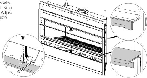
3. Install the left (L) and right (R) trims with the flanges facing outward. Adjust the trims to the desired depth and tighten the screws and shoulder bolts.
