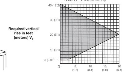
Horizontal vent run plus offset in feet (meters) H<sub>-</sub> The shaded area within the lines represents acceptable values for  $H_{\scriptscriptstyle T}$  and  $V_{\scriptscriptstyle T}$
