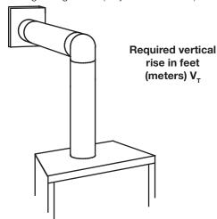
See graph to determine the required vertical rise  $V_{\scriptscriptstyle T}$  for the required horizontal run H<sub>+</sub>.
