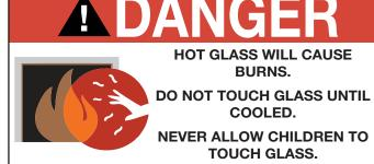
A barrier designed to reduce the risk of burns from the hot viewing glass is provided with this appliance and must be installed for the protection of children and other at-risk individuals.
