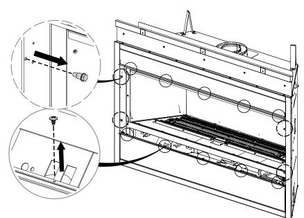
2. Install the top 1" (25mm) trim and bottom 1 1/2" (38mm) trim with the flanges facing outward. Note the orientation of the trim. Adjust the trims to the desired depth.
