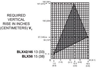
HORIZONTAL VENT RUN PLUS OFFSET IN FEET (METERS)  $\mathbf{H}_{\mathsf{T}}$ The shaded area within the lines represents acceptable values for  $\mathbf{H}_{\mathsf{T}}$  and  $\mathbf{V}_{\mathsf{T}}$
