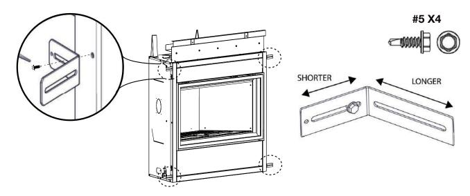
Use one screw to secure the short side of the nailing bracket to the appliance. Repeat for 3 other locations.
