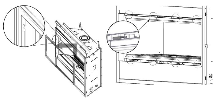
Before the glass door can be removed, the safety barrier must be removed. Lift the safety barrier off the four shoulder screws and remove from the appliance.
