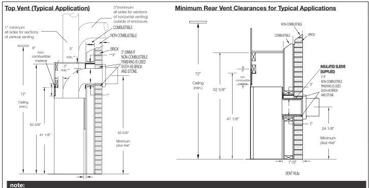
Vent Sections: When passing through a wall, use the appropriate firestop spacer W010-4479 (not supplied) for flex venting or 5DHFSN (not supplied) for rigid venting. When passing through a ceiling, use firestop spacer W500-0028 (not supplied) for flex venting or 5DFS (not supplied) for rigid venting. For venting and minimum clearance to combustibles, refer to appliance manual.
