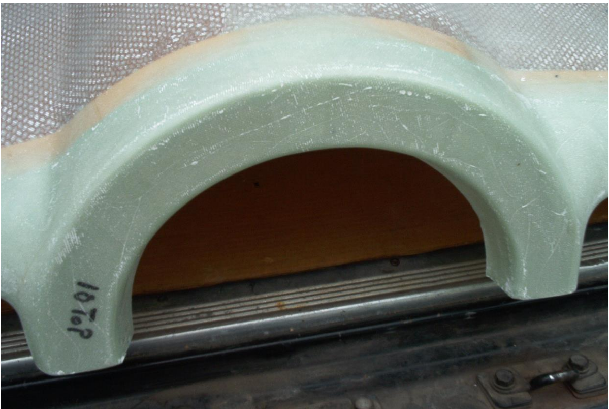
Photo 2 – Loehle Wonder-Fil showing pinholes in honeycomb areas on RV-10 cowling.
