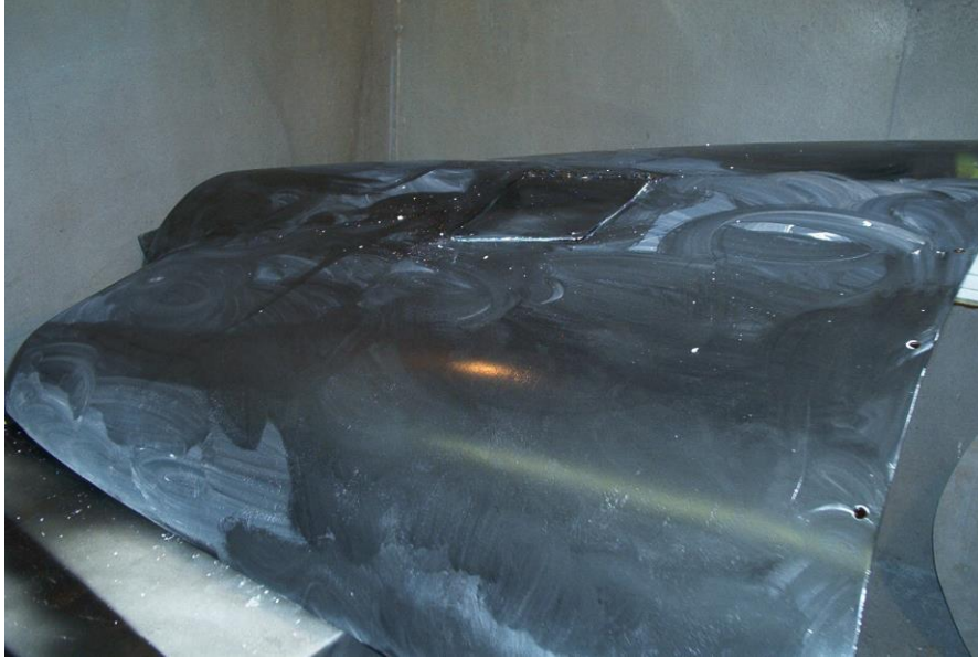
Photo 4 – Whitish haze shown on upper cowling before wiping off surface with towel.
