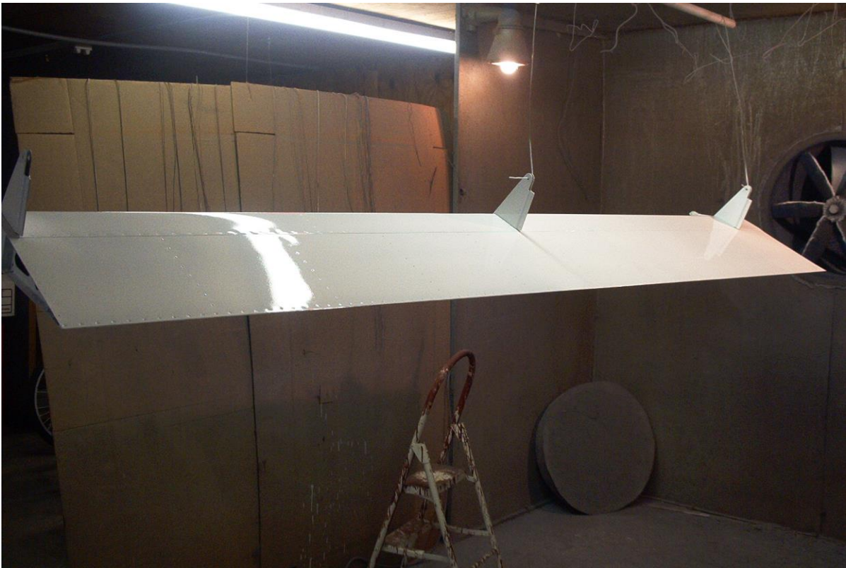
Photo 20 – RV-10 flap with White Color Top Coat applied over White UV Blocking Primer .
