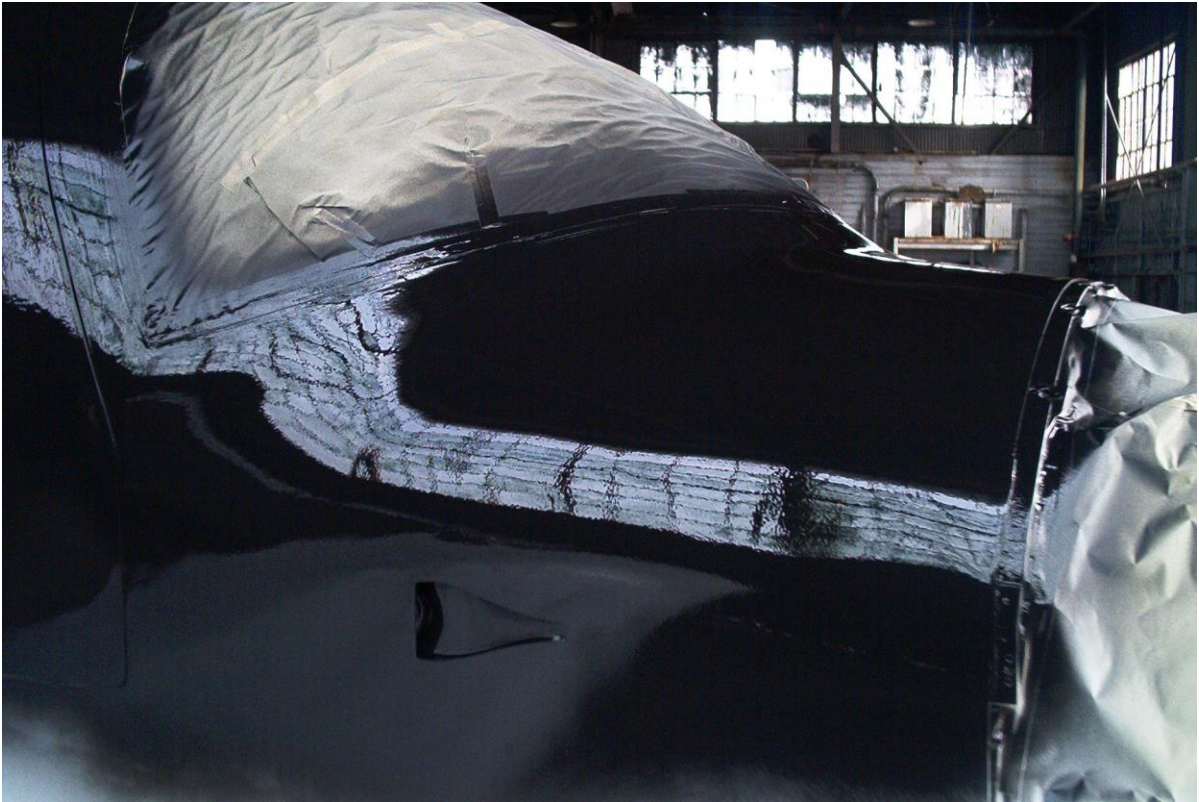
Photo 7 – Shiny finish of Black UV Blocking Primer before sanding windshield area on RV-10.
