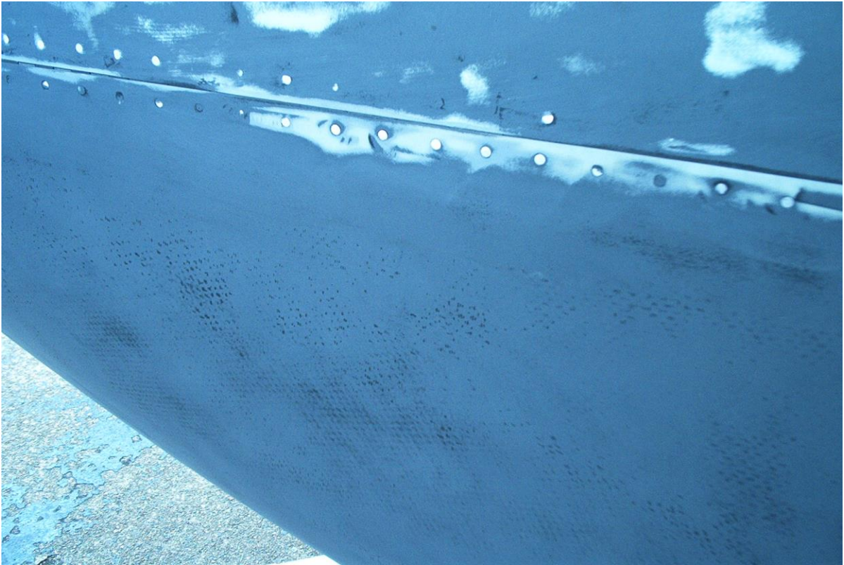
Photo 6 – Fabric weave and honeycomb lamination clearly shows up after applying Black UV Blocking Primer coating. Additional Black will fill in these areas.
