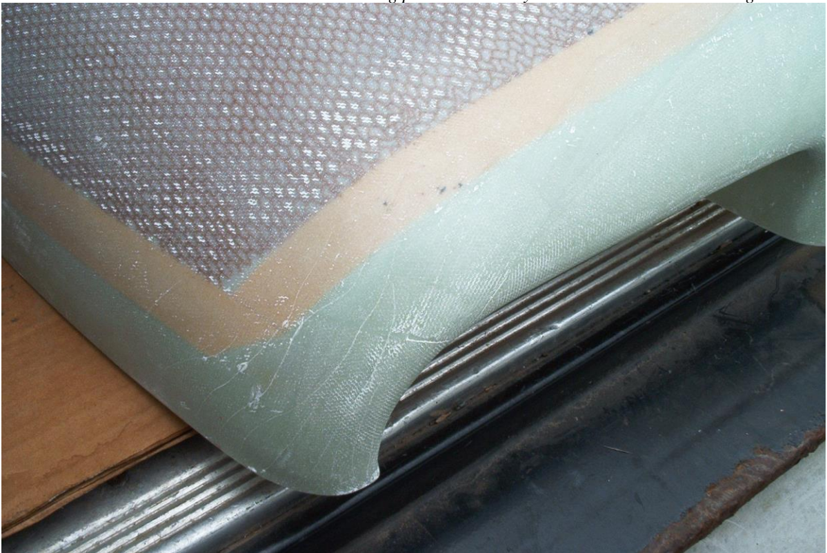
Photo 2 – Loehle Wonder-Fil showing pinholes in honeycomb areas on RV-10 cowling.
