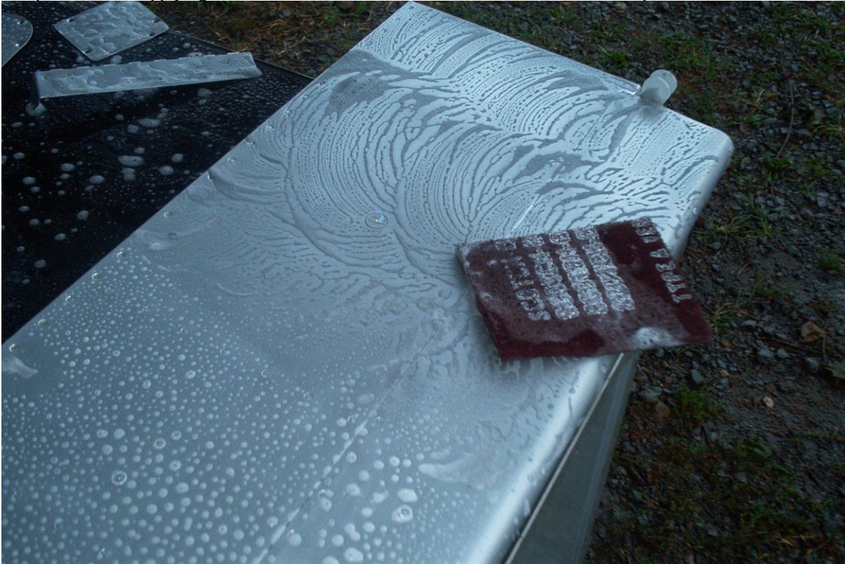
Photo 19 – Scuffing surfaces with abrasive pad. This is typical of initial scrubbing with detergent and when applying Aluminum Etch , Alodine or Pre-Kote. The surface MUST NOT bead up water or it's not scuff sanded enough.
