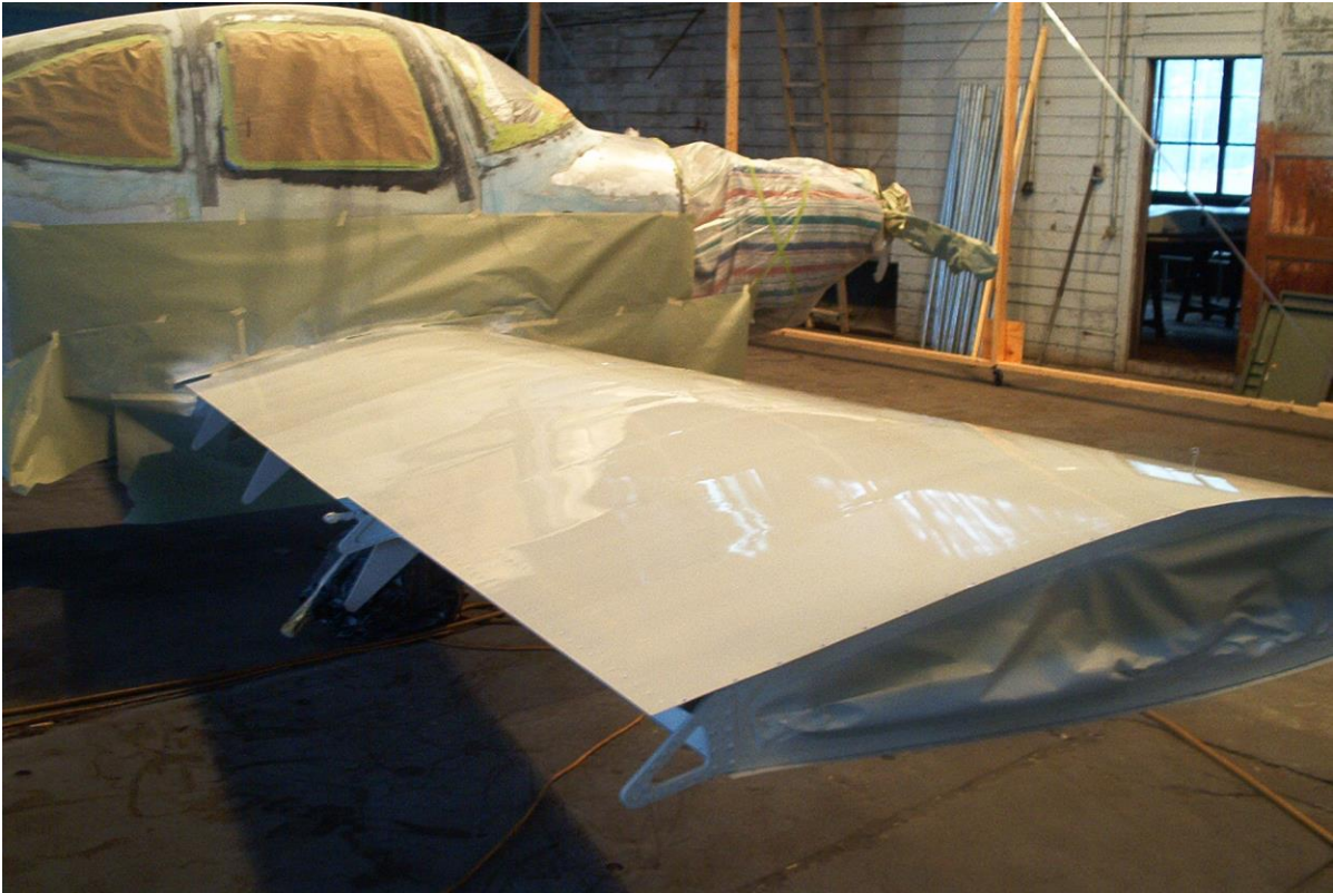
Photo 16 – White UV Blocking Primer applied to all metal wing of RV-10.
