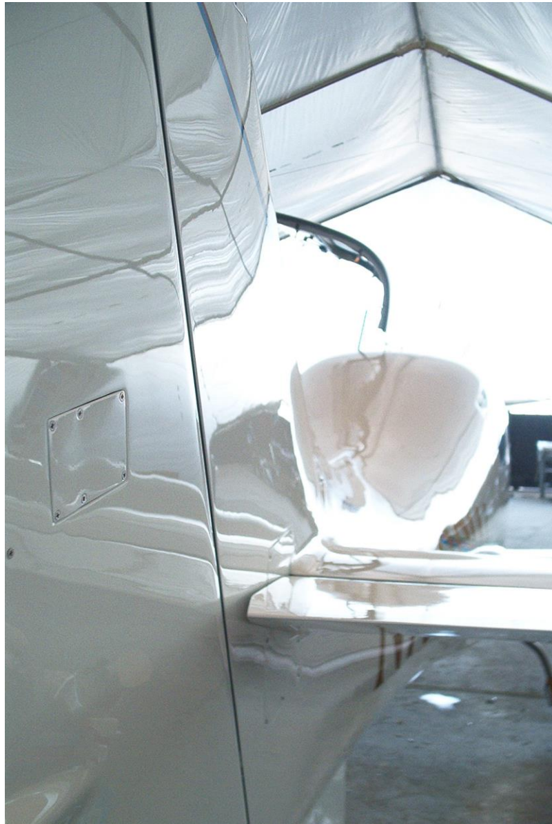
Photo 25 – Final buffing of Lancair IV Propjet fuselage...shiny curves galore!
