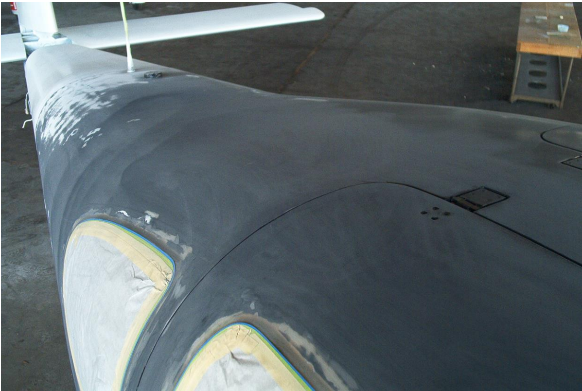
Photo 11 – Smoothly sanded upper cabin area of RV-10.
