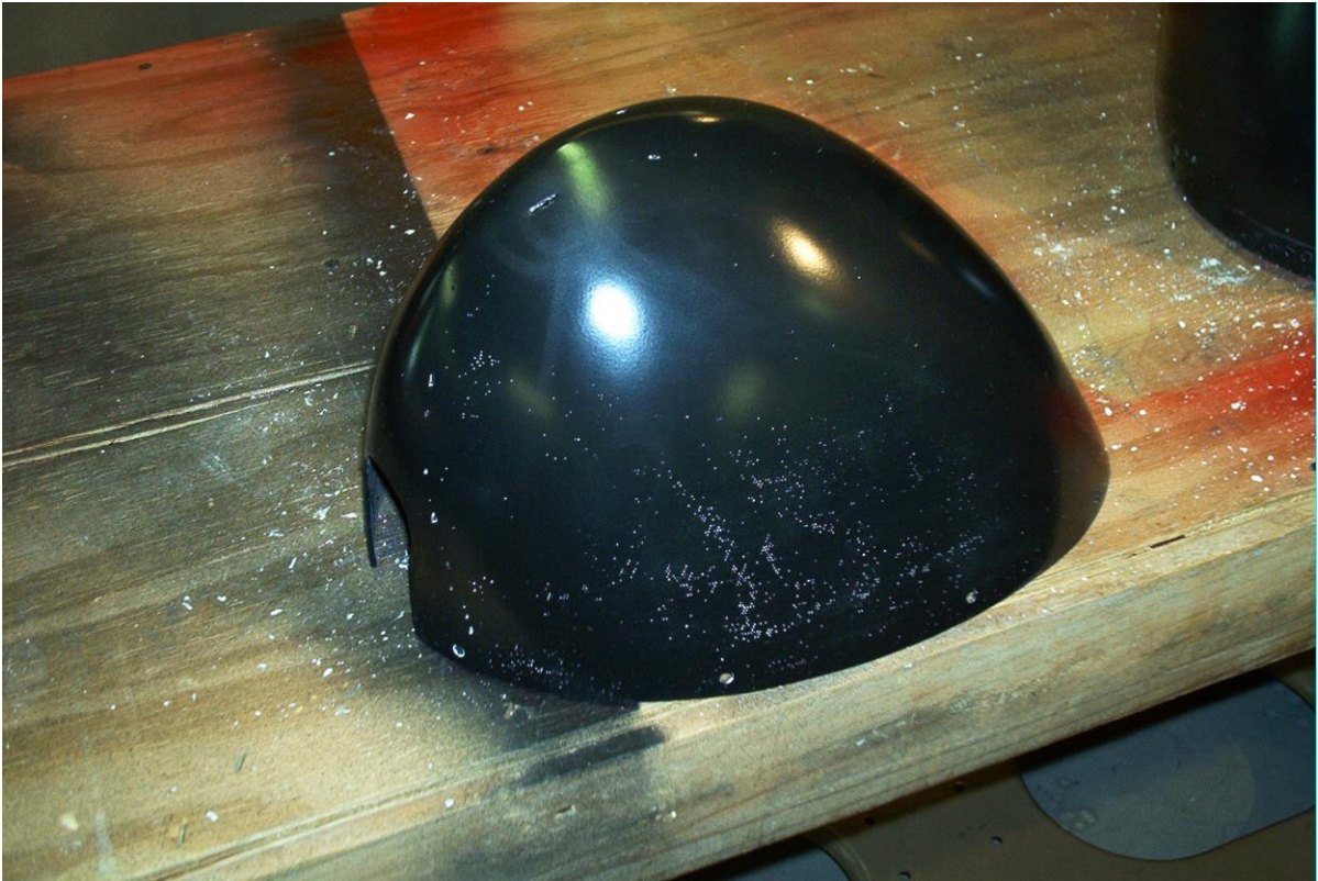
Photo 5 – RV wheel pant nose with Black UV Blocking Primer sprayed on before any Wonder-Fil was used – pinholes really show up then!
