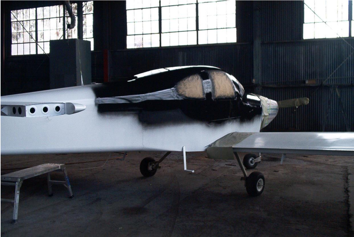
Photo 17 – Black UV Blocking Primer used to achieve smooth blends of composite areas to metal area.
