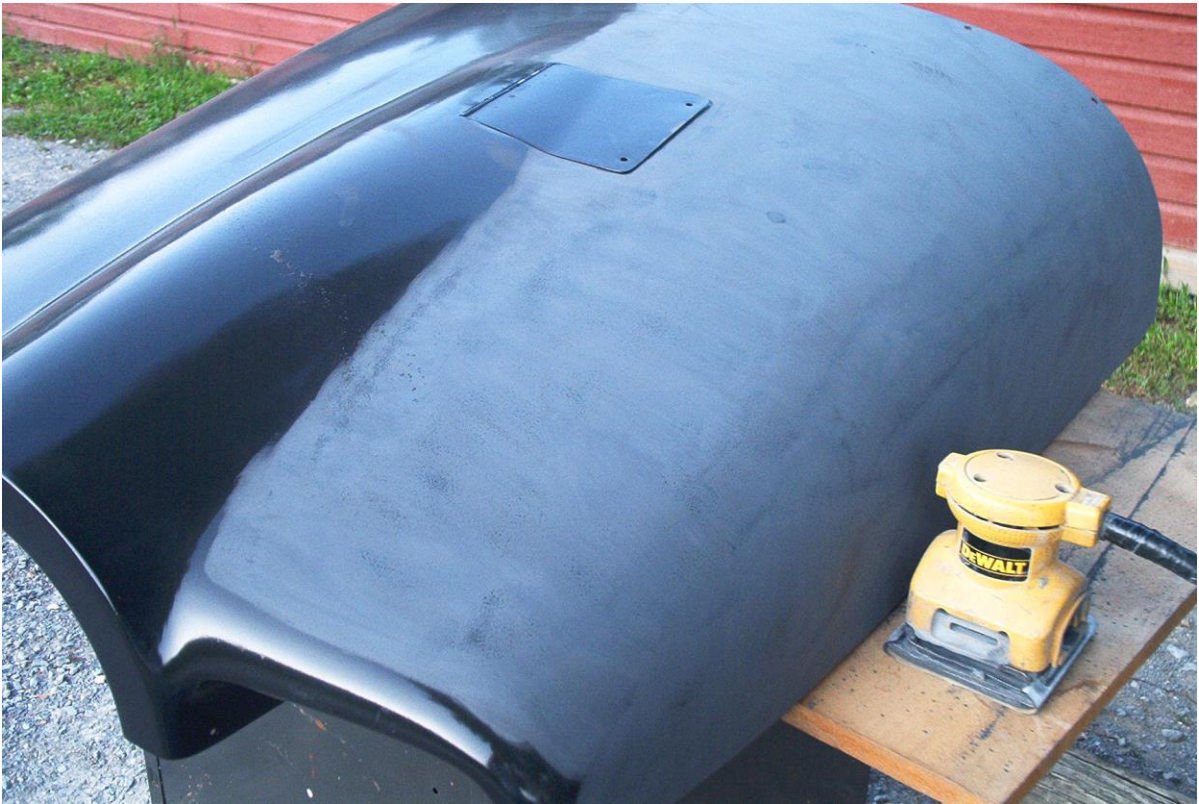
Photo 8 – Obvious comparison of sanded and unsanded Black UV Blocking Primer on upper half of RV-10 cowling.
