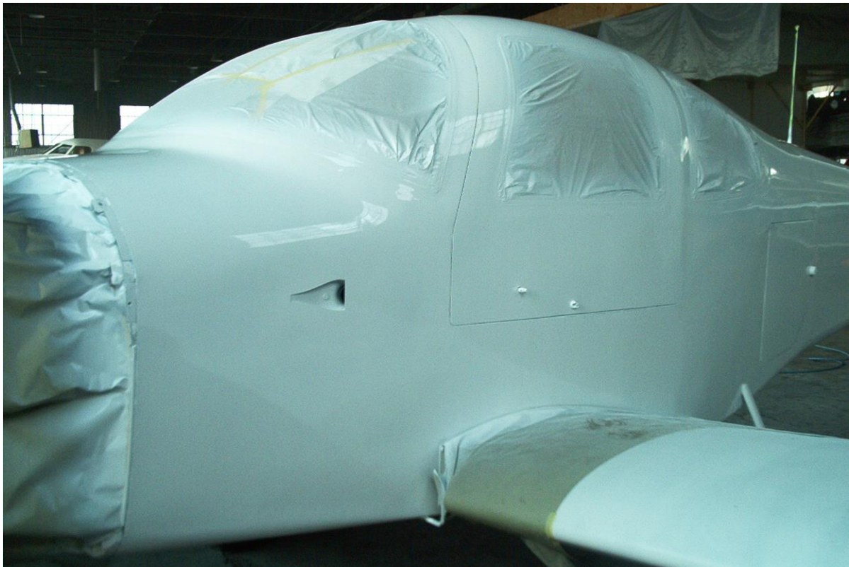
Photo 15 – White UV Blocking Primer sprayed over smoothly sanded Black coats.
