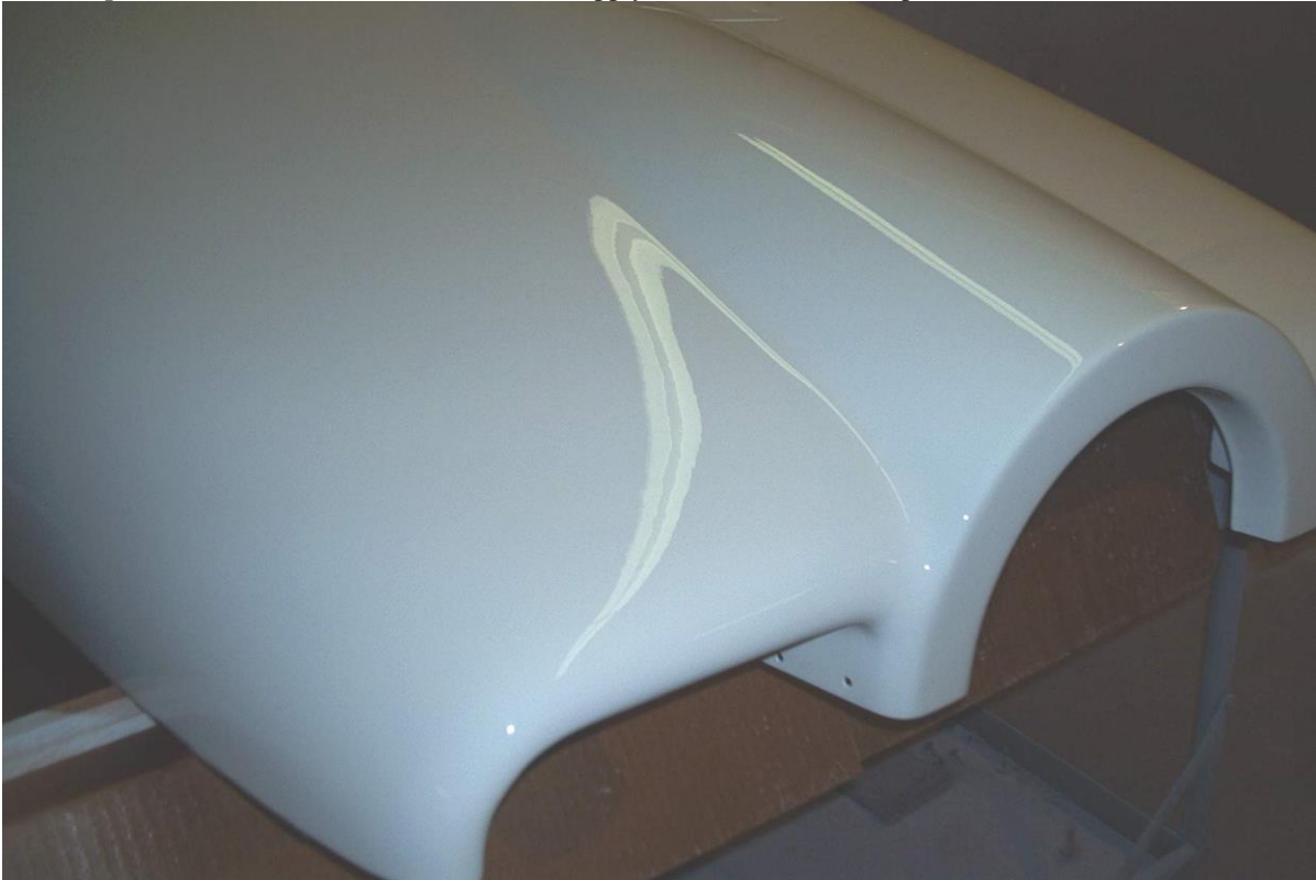
Photo 24 – High gloss unpolished shine of Clear Top Coat applied to upper RV-10 cowling.
