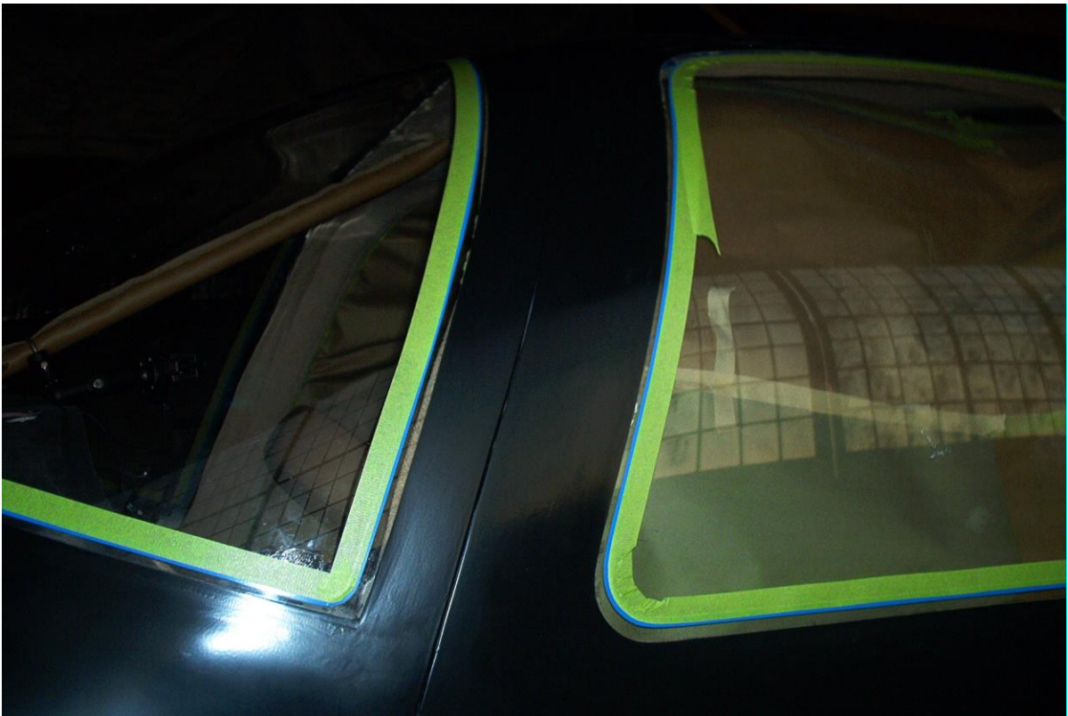
Photo 21 – Blue plastic finishing tape applied to windshield for perfect paint line. Good quality paper tape is butted next to the plastic tape.
