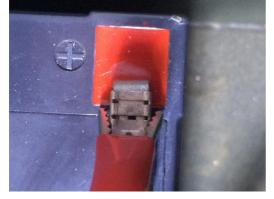
5. The clamps when attached correctly:
