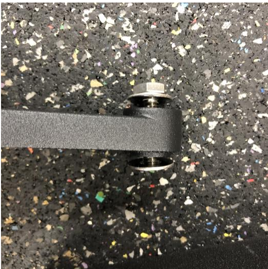
USE THE SMALLER BOLT FOR THE MOUNT. ONE WASHER SHOULD BE USED ON BOTH SIDES OF THE MOUNT
