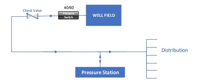
Pressure Station consists of as many as 9, 119 gal pressure tanks (AMTROL WX-350), providing ≈ 400 gals before asking for water from the well. Water supply & distribution mains might be as small as 4-inch with 1-inch takeoffs.
