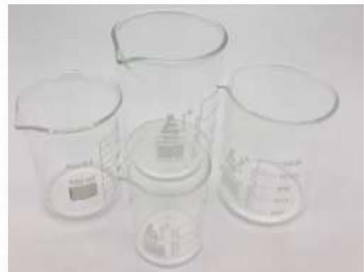
**GLASS POURING BEAKER HANDLES** – Handles are designed to easily and quickly slide onto beaker to aid in pouring. Do not use handles when heating resin in microwave or over stove. Simply slide onto beaker after heating resin. We recommend having the beakers ready with handle installed then pouring heated resin from another container into beaker when ready to pour.
