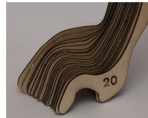
Bench profiles of 12mm Plywood will be cut using a CNC machine, having 3 profiles fit into 2 plywood sheets. The cut profiles will be primed and painted. Within the profile holes in each plywood profile will be set in key points where the threaded bar will go through the entirety of the bench.
