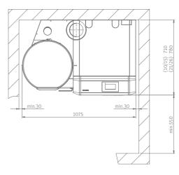
\*Minimum clearance with rear vertical flue pipe conncetion upwards is 350mm.
