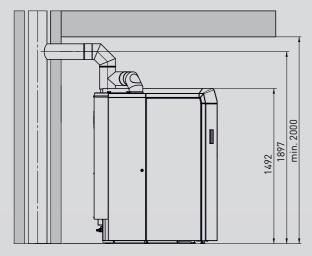
Minimum clearances DuoWIN Flue gas collector set DUO 002 vertical installation
