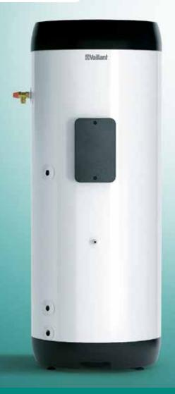
The standard uniSTOR heat pump cylinder is available in 150, 200, 250 and 300 litres. Each cylinder uses the latest thermal injected insulation for the lowest heat losses in its class, with as little as 1kW per 24 hours. The strategically positioned large diameter, smooth coil provides optimum hot water performance and automatically de-scales to ensure long term efficient hot water generation.
