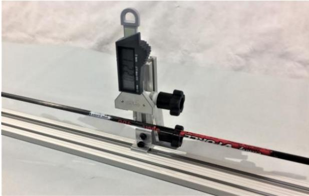
Position the gauge so it's in the center of the shaft with about  $\frac{1}{2}$  inch of the pointer showing.
