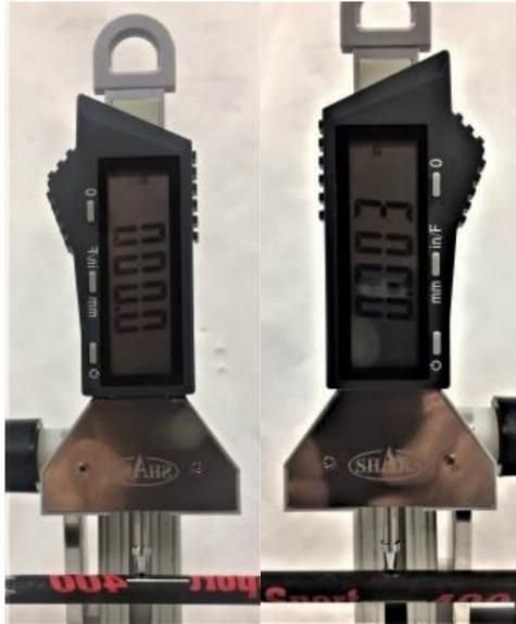
Zero the gauge and rotate the shaft. If the gauge shows a negative value stop it on the highest number and re-zero. This will make reading easy. Now rotate and watch.
