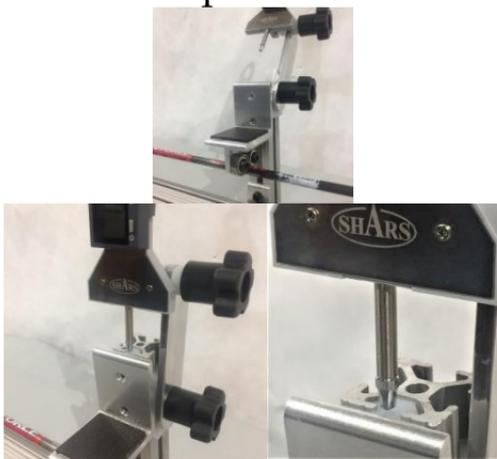
Position the gauge so the pointer sets squarely on the nylon guide and lower into position so that it is approximately  $\frac{1}{4}$  in from the nylon guide. Turn on the gauge, set to inches and push zero to reset, as shown in picture.
