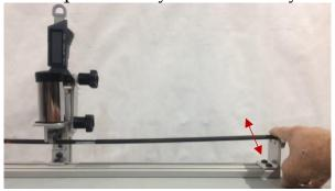
With the weight on the pan simply roll the shaft. You will feel it roll into a valley. It's easier to apply a little more weight to the pan by pushing the weight down with your left hand and rolling the shaft with your right.
