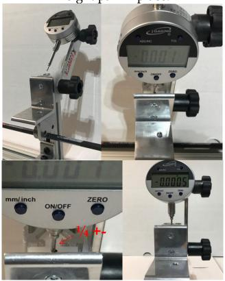
Position the gauge so the pointer sets squarely on the nylon guide then lower into position so that it is approximatly  $\frac{1}{4}$  in from the nylon guide. Turn on the gague, set to inches and push zero to reset, as shown in picture.
