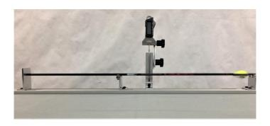
Roll the shaft with your left hand keeping the point against the target
