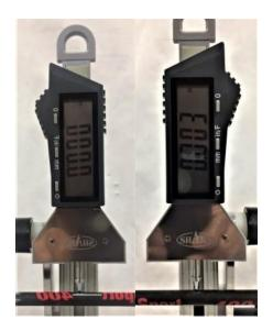
Zero the gauge and rotate the shaft. If the gauge shows a negative value stop it on the highest number and re-zero. This will make reading easy.
