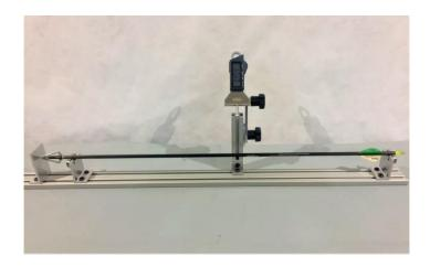
Tape a piece of paper to the target and mark the point where the shaft touches the paper. Rotate the arrow and watch for tip movement. If the point makes a circle, tweak tip until perfect.
