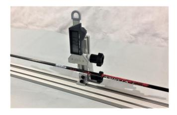
Position the gauge so it's in the center of the shaft with about a ½ inch of the pointer showing.
