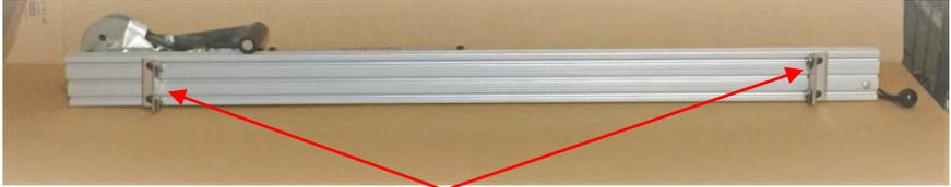
slide the 2- 3 inch brackets on the back of the machine and tighten in place.
