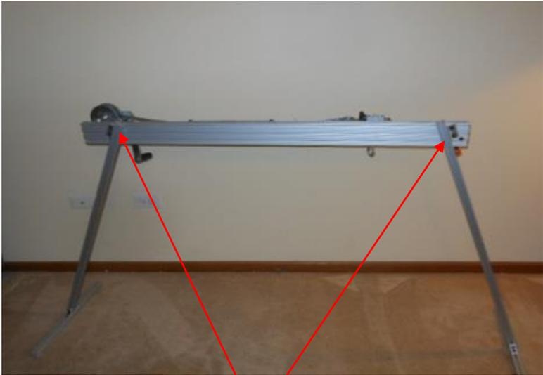
*Slide the legs into the 3 inch brackets on the back of the draw –board as shown in the pics*
