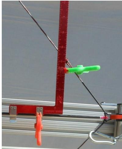
Measure from the center of the shaft to the center of the peep and slide the parting string to the exact spot to where the peep will go.
