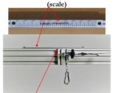
The linear guide block will line up with the draw length. If you're hooked to the D - loop it will give you your draw length including the D-loop NOTE: scale may need to be adjusted to proper draw length.
