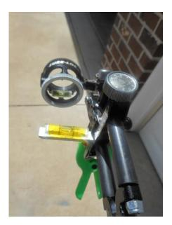
Figure 66 Now with the elevation slide plumb to the riser, it's time to set your sight bubble.
