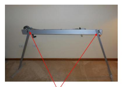
Slide the legs into the 3 inch brackes on the back of the draw –board as shown in the pics
