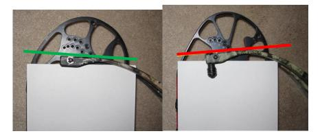
Almost parallel + 1 Past-parallel - 6 degrees degree Almost Parallel versus Past Parallel
