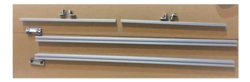
The leg kit is in the white box. It contains 2-3 inch brackets that mount on the back of the machine. 4 -1- inch brackets that mount the ½ feet to the legs.
