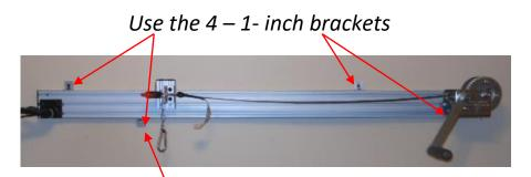
Slide inside the top and bottom and align to your wall studs and screw in place with the appropriate drywall screws.
