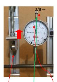
With the rollers positioned up and out of the way position the dial indicator against the shaft so as to have an adequate amount of movement.
