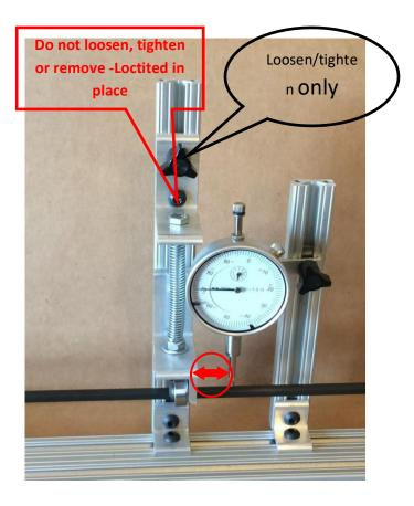
NOTE: keep the dial gauge close to the pressure point. Testing has shown no measurable distance in deflection when kept to a minimum.
