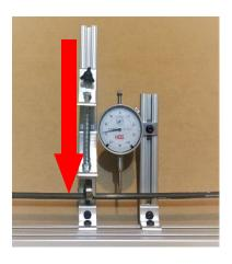
Apply enough downward pressure to rotate the pointer 2 to 3 times and lock in place and rotate dial face so 0 is once again centered on the pointer.
