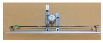
Center of the shaft should be centered between the dial gauge and the spring loaded rollers
