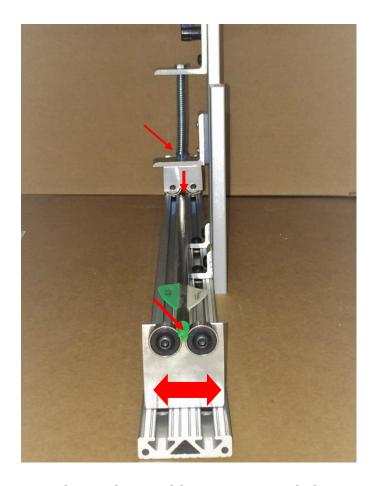
Adjust the end bearings until the center press lines up on the center of
