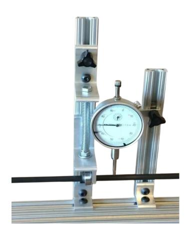
NOTE: keep the dial gauge close to the pressure point. Testing has shown no measurable distance in deflection when kept to a minimum.
