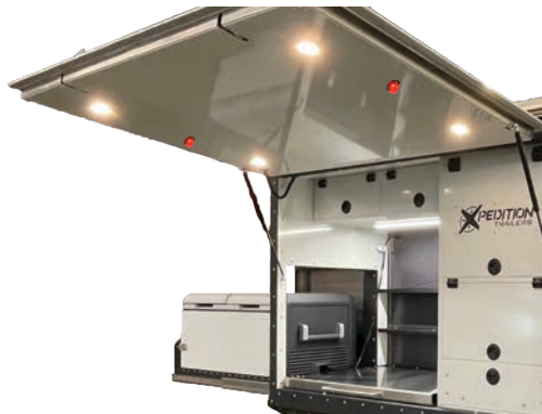
Underside Back Door Red Area Lights
