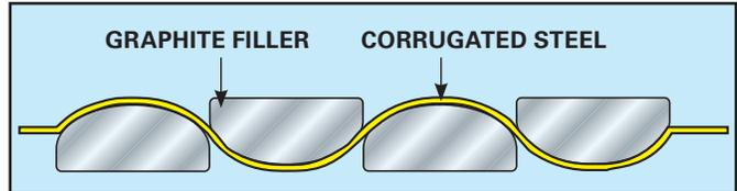
Standard corrugated steel gaskets without graphite as specified in API 600 were found to be an unacceptable choice for low emission service, even under ideal laboratory test conditions, and regardless of the flange finish and gasket load. After testing several alternative gaskets, we selected the best performing gasket in our tests—a corrugated steel gasket with graphite-filled channels.
