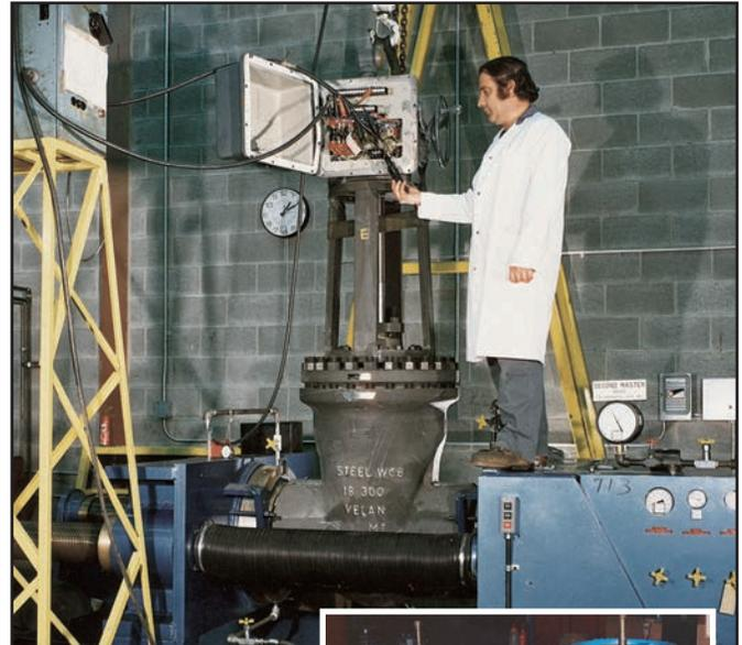
Above: Operational test for electric actuators.
