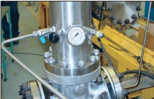
*A global measurement technique used by ISO 15848-1 provides highest sensitivity to leakage.*
