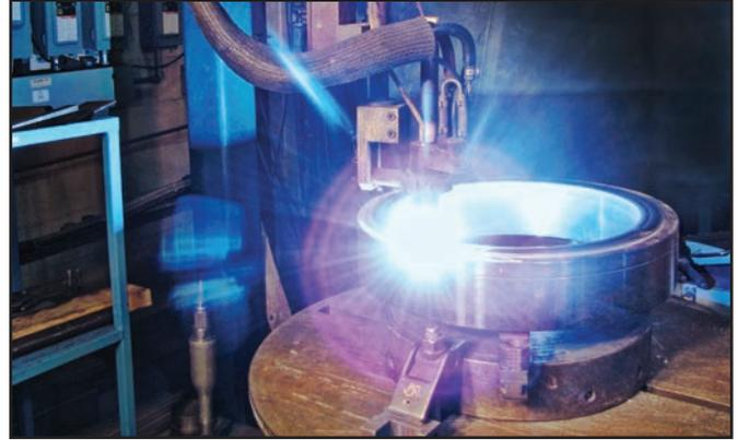
Automatic plasma arc hardfacing equipment for seats.
