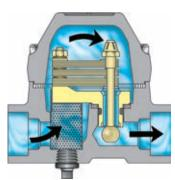
This is the first step in the smooth and quick opening of the valve, without noise or violent action. When the flow is released, the unbalanced pressure acts on the full valve area. The force to overcome the thermal pull increases and opens the orifice to full capacity.
