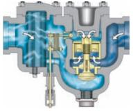
When pressure is off, equipment discharging to a
