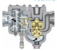
When condensate is discharged, the float mechanism rests on the trap body. The bimetal element alone, closes the valve with thermal power developed by incoming steam. The bimetal element is a function of the saturated steam curve, therefore operates efficiently at any pressure within it's range.
