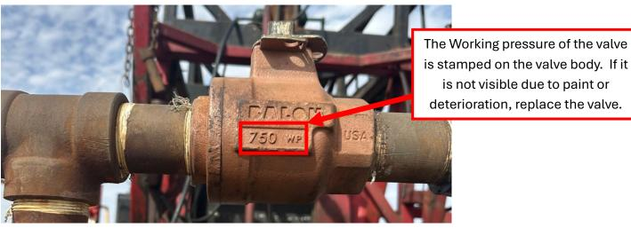
is stamped on the valve body. If it is not visible due to paint or deterioration, replace the valve.
