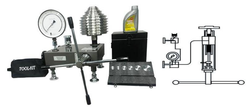
Models of DW 10 series are provided with one large capacity screw pump and a removable oil reservoir with isolating valve in a simple line circuit permitting effective air removal.
