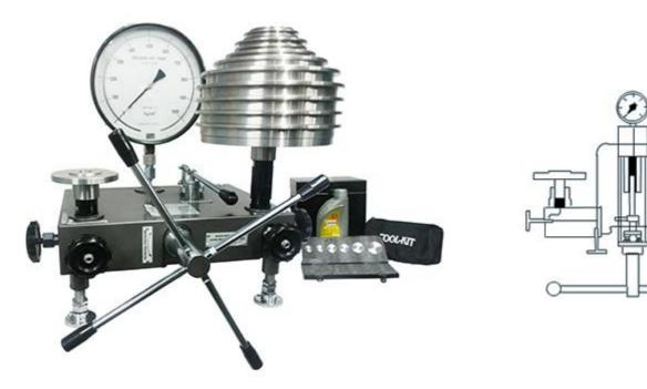
Models of DW 30 series are provided with 2 free piston assemblies for giving Low Pressure range with smaller steps and High Pressure range with larger steps in a single instrument with substantial cost saving. The ratio of areas of LP and HP Free Pistons is generally 10:1. Ratio of 5:1 or 20:1 can also be provided.
