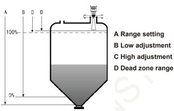
The reference surface for measurement is: the bottom surface of the thread or the sealing surface of the flange. Note: When using radar level timing, it must be ensured that the highest material level cannot enter the measurement blind zone (the area shown by D in the figure).
