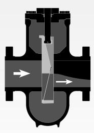
During travel towards the open position, the gate slides across the wedge angle of the segment, collapsing the assembly so that it travels freely between the seal faces. The patented Leverlock gate centralizer holds the mechanism in the neutral position until seal expansion is required.
