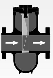
When the bore in the segment is aligned with the conduit bore, an end-stop prevents further travel and the gate slides across the wedge angle, expanding the gate and the segment, isolating the flow from the body. The preferred flow direction assures easier operation.
